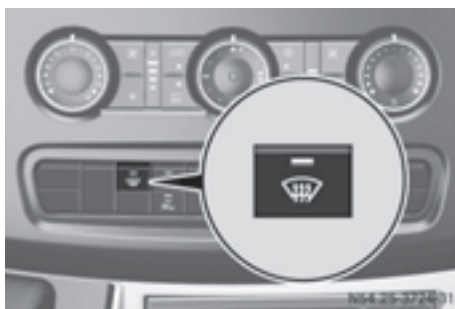
Windshield heater switch
