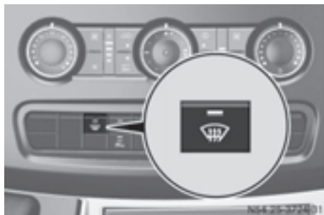
Windshield heater switch
