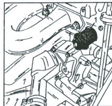
Fig. 1.66 – The chain tensioner (1) is located at the side of the engine.
