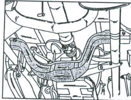
Fig. 1.5 – The attachment of the crossmember underneath the vehicle.
