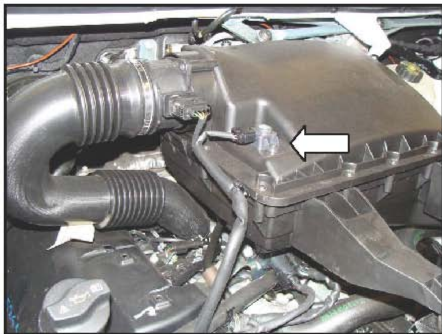
B28/19 - Pressure sensor downstream of air filter
