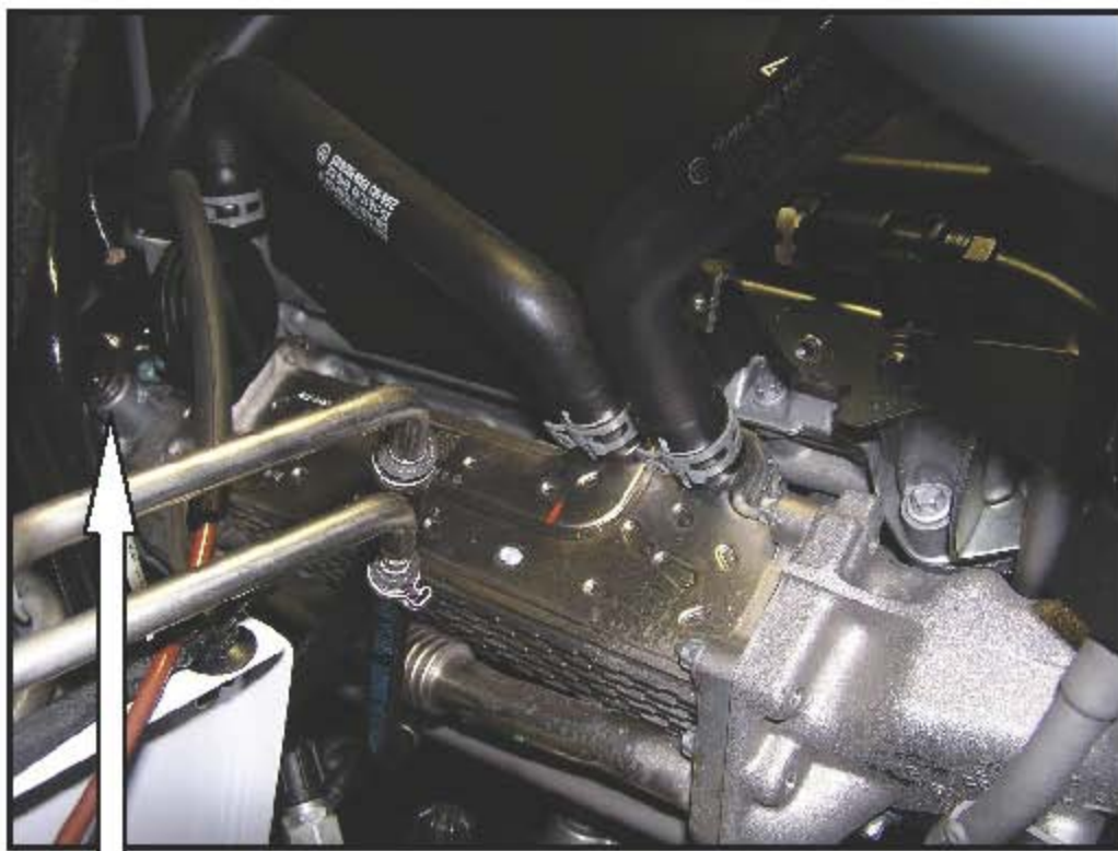
B60/4 – At rear of EGR cooler
