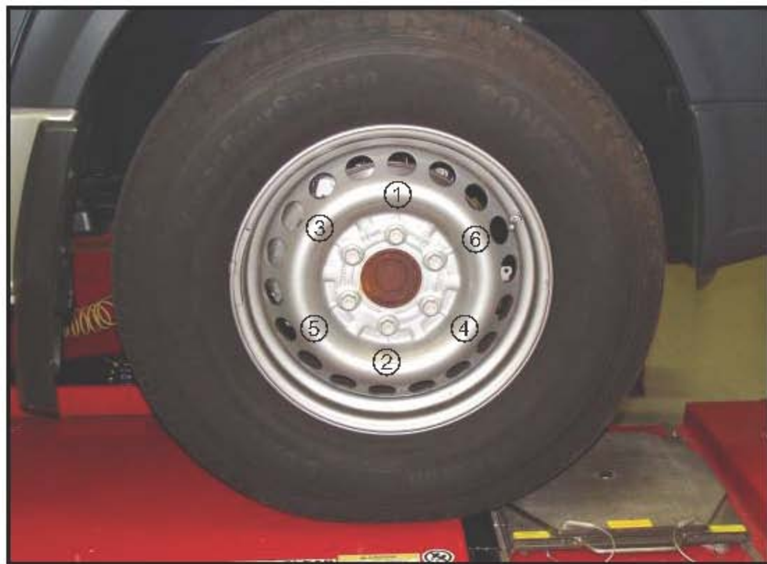
Tightening Torque Pattern
